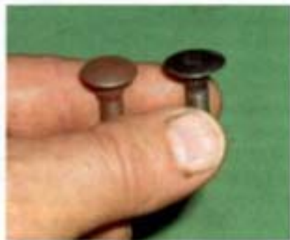
Note the difference in the head shape and collar shape between the American bolt (left) and the French bolt. My friends both in France and the U.S. held me to my word of an accurately recreated ambulance.
