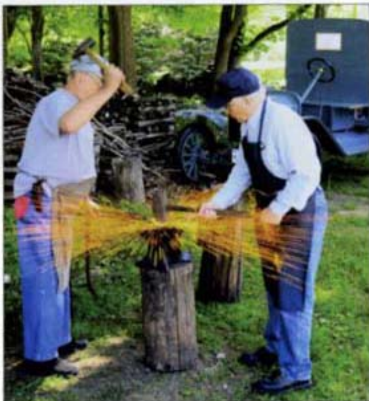
Sparks fly as Ted and George forge one of the larger pieces for the tailgate of the ambulance
