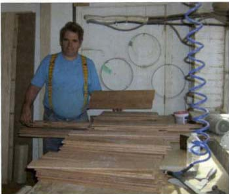
Matt Malley of H&B Woodworking making the eighty-six mahogany, tongue and groove boards for the sides and front of the ambulance body.
